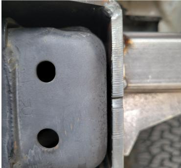
Make sure everything lines up, the pin goes in the hole and the latch lines up to the hook.
