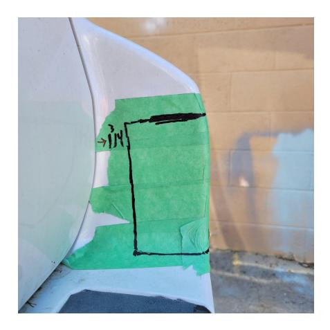
Once you've marked out the cut out with the measurements provided in the image above, use any tool you see fit for the job to do the cut.
